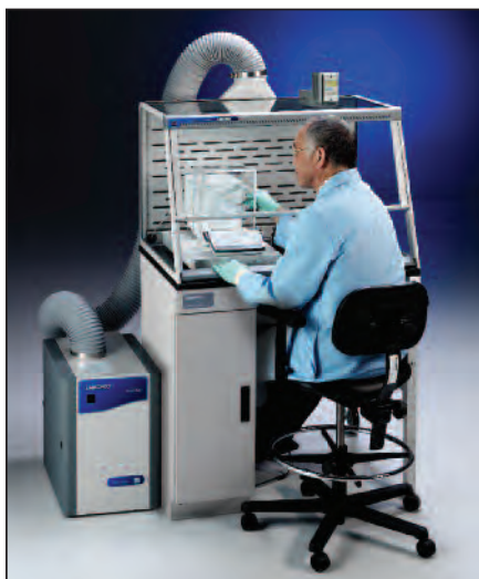
The XPert Easy-Order includes the XPert Balance Enclosure, Black Solid Epoxy Work Surface and FilterMate Portable Exhauster. Supporting base is not included.
